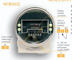
The device with HART output can be connected to a PC using a SAT-304 HARTUSB modem. All the data measured by the **AnaCONT** can be seen on the PC, and if needed the transmitters can also be programmed from here. Max. 15 normal (non Ex) instruments can be connected to a HART line. Applicable softwares: **EView** configuration software or **NIVISION** process visualization software.
