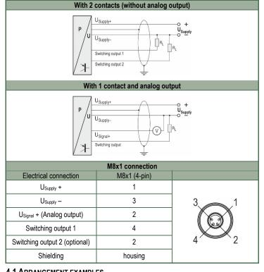
Use a shielded and twisted multicore cable for the electrical connection.
