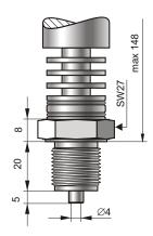
**RG type** G1/2" with radiator **RM type** M20×1.5 with radiator
