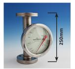
MT meters are installed in vertical lines with flow upwards and are normally supported by the pipework.
