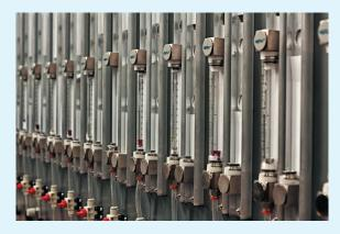
Each flowmeter scale is produced using our bespoke air or water calibration facilities where all reference equipment used is traceable to national standards and controlled within our approved ISO9001:2008 management system, assuring accuracy within the required limits.
