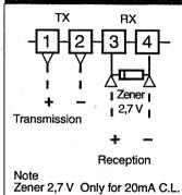
Interface 20 mA C.L. passive and galvanically isolated
