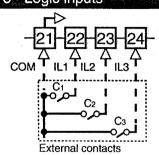
The permanent closing of the external contacts C1, C2, C3 allows:
