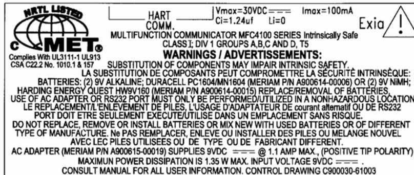
**WARNING:** *Serious injury or death may result from explosions. Do not make connection to the DB – 9 connection port or to the AC adapter jack while in a hazardous area.*
