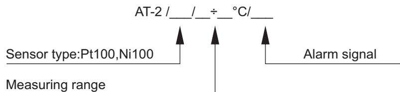
Example: temperature transmitter AT-2, sensor type Pt100, measuring range 0...100°C, alarm signal 22mA.
