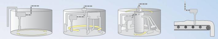
In a rotating pan mixer or conveyor application, the Hydro-Probe Orbiter can be cabled directly to the control system. In a static pan mixer the sensor cable is routed through the Hydronix Rotating Connector.
